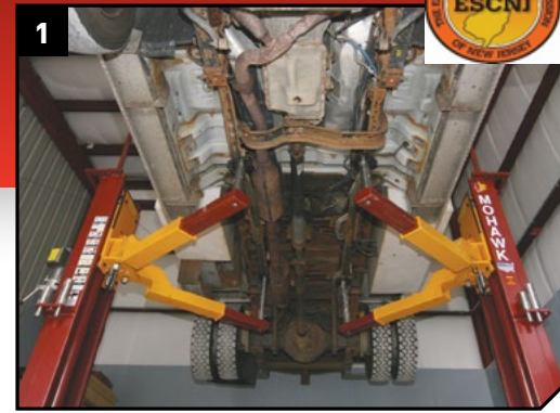
▲ Two post lifts offer FULL unobstructed under vehicle access for all repairs, take up minimal bay space and leaves wheels hanging free for tire, brake or any other necessary repairs.
