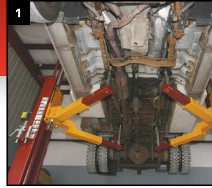
▲ Two post lifts offer FULL unobstructed vehicle access for all repairs, take up minimum space and leaves wheels hanging free for tire or any other necessary repairs.
